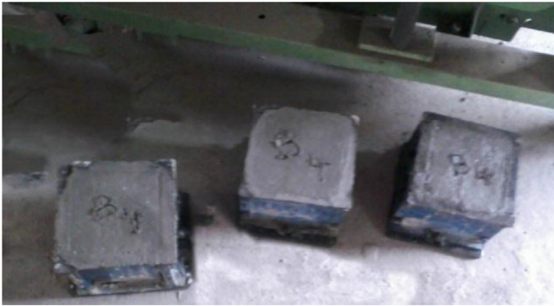
Fig. 2. Concreting of Cubes.
