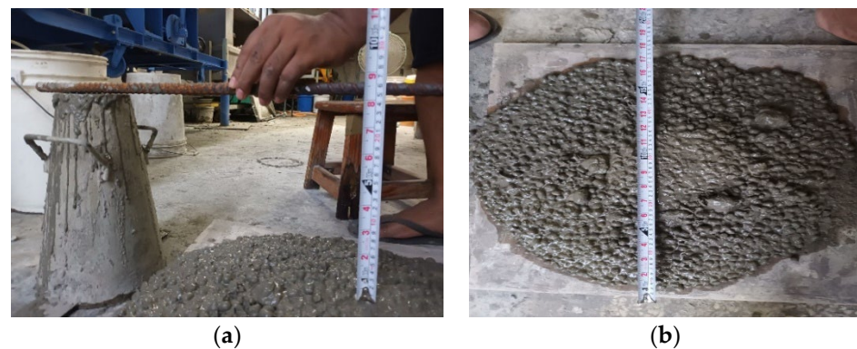
Figure 3. Slump cone test (height = 24.2 cm and slump flow diameter = 51 cm).
