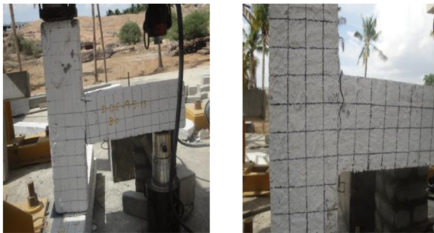
Fig. 8. Crack Pattern of Control and Basalt Fiber Reinforced Concrete Beam-Column Joint Specimens.
