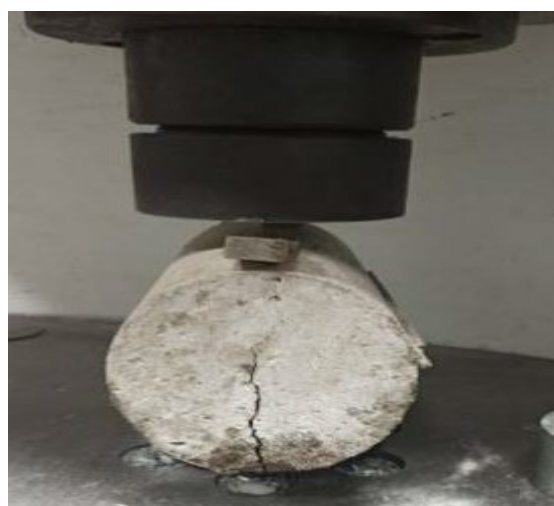
Figure 6. Split tensile test of the cylinder.
