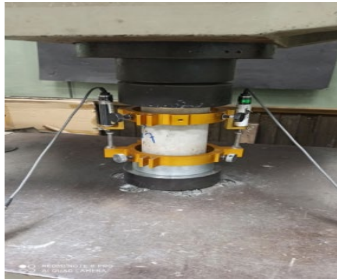
Figure 4. Cylinder compressive strength test with LVDT.
