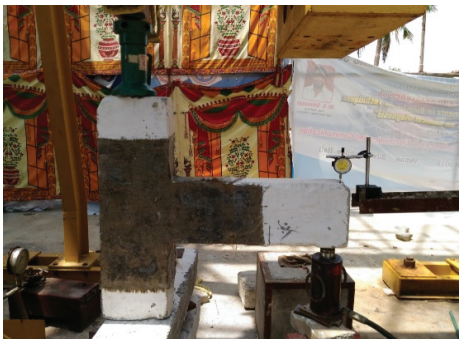
Fig. 6. Reverse loading arrangement of beam column joint
