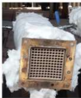
Figure 6(a). Pictorial View of 8mm honeycomb SCR type catalyst
