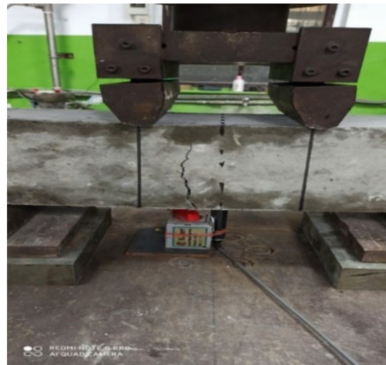
Figure 7. Flexural test of beam specimen (four-point loading).
