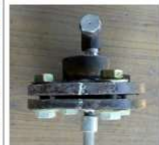
Fig 9 (b). Ammonia Injection Nozzle
