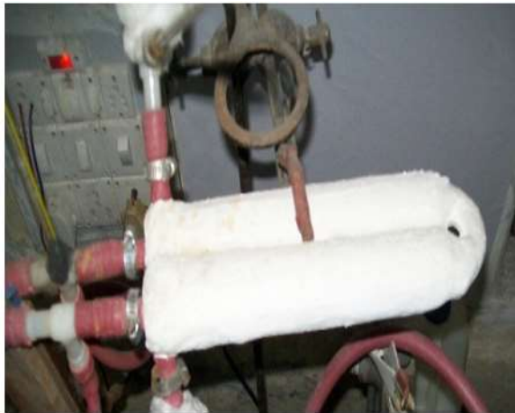
Figure.: Installed miniature double tube Hairpin heat exchanger in laboratory.
