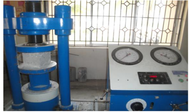
Fig. 5. Test setup of Cube Compressive Strength.
