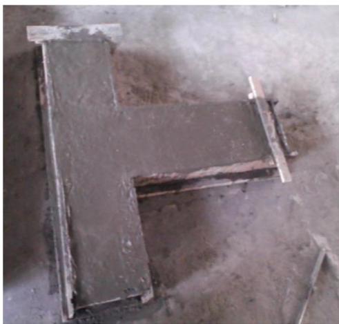
Fig. 4. Casting of Beam - Column Joint Specimen.
