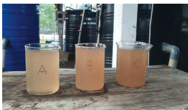
Diluted Soak Effluent at 15,000 TDS Diluted Soak Effluent at 25,000 TDS Raw Soak Effluent at 35,000 TDS
