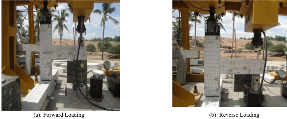
Fig. 6. Experimental Test Setup of Beam-Column Joint Specimen.
