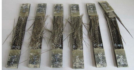
Fig. 3. Failure patterns of basalt fabric sample
