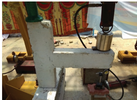
Fig. 7. Forward loading arrangement of beam column joint
